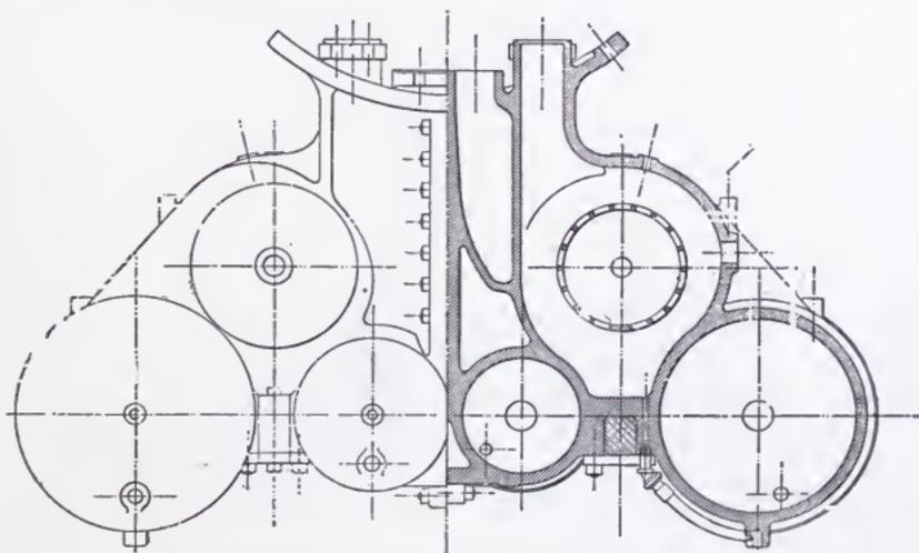
CROSS SECTION OF BALANCED COMPOUND CYLINDERS
