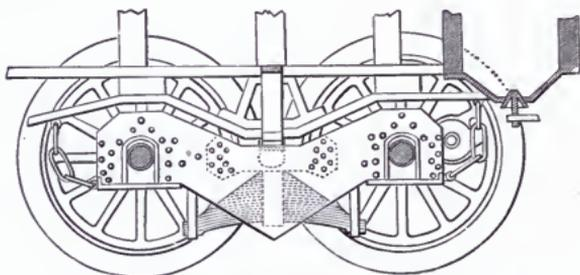
BALDWIN FLEXIBLE BEAM TRUCK, 1842—ELEVATION
