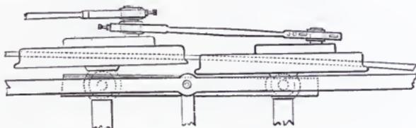
BALDWIN FLEXIBLE BEAM TRUCK, 1842—HALF PLAN
